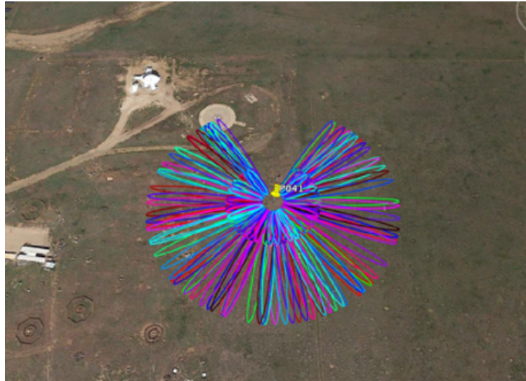
Figure 7: Illustration of ground reflections in the surroundings of the receiver antenna.
