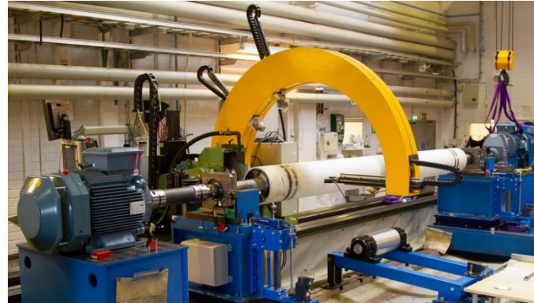
A rotor test rotor ecosystem: force and acceleration measurement at both bearings, 4-point roundness and center movement measurement, adjustable foundation stiffness and external loading systems,
