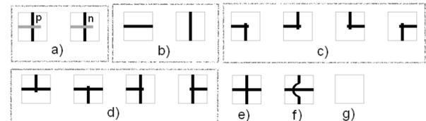
The marks on the tiles indicate the arrangements of the SWNTs affixed on the respective DNA origami: a) p-type and n-type CNFETs, b) straight CNWs, c) corner CNWs, d)-e) 3- and 4-way CNW junctions, f) crossing but non-interacting CNWs, g) blank tile (used for analyzing fault tolerant architectures).
