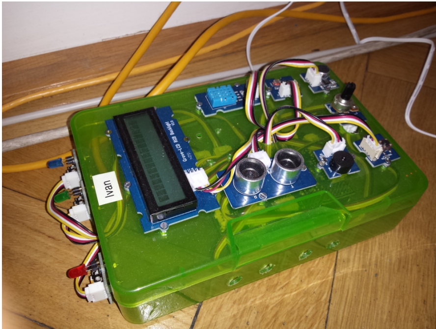
Figure 7.7: An example of our gateways for Building Management Systems.
