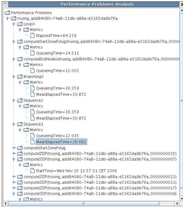
Fig. 14. Example of performance problems detected in the CTM workflow. Nodes under the tree root represent instances of workflow, workflow regions and activities. Under a node representing an instance is a subtree visualizing performance metrics.
