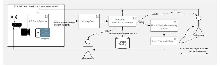
Fig. 2. IoT & Analytics for Predictive Maintenance
