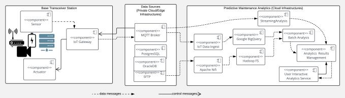
Fig. 1. BTS, data sources and services for predictive maintenance
