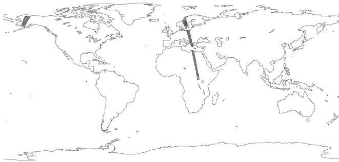
Fig. 4. The ground track—restricted to the Land Masses acquisition region—along which simulated 1 minute DEM-geocoded IW mode GRD slices at 1 km resolution were generated in support of evaluating the timeliness of the S2M-NRT.
