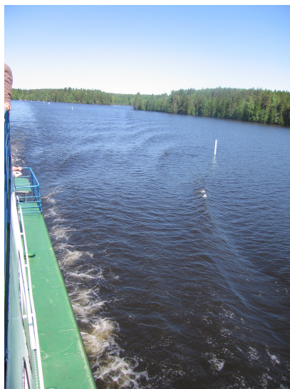
FIG. 1: Waves formed by a ship on a lake at the Saimaa canal.
