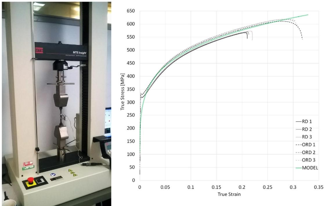
Figure 1: Tensile testing equipment and test results in the rolling direction (RD) and orthogonal to rolling direction (ORD).
