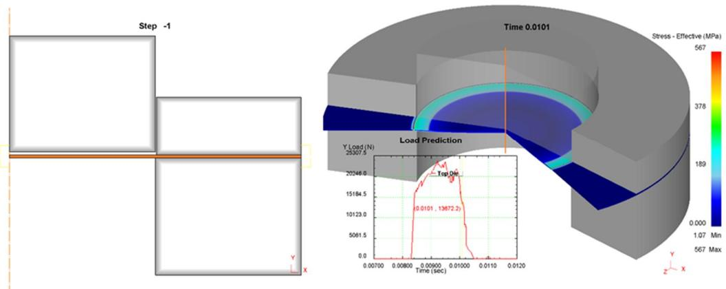
Figure 4: Axisymmetric 2D simulation setup for hole piercing.
