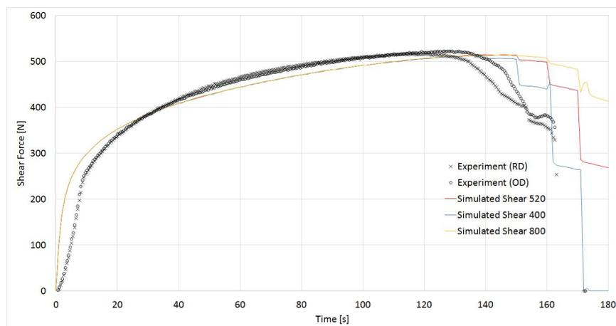
Figure 6: Shear force from simulations (red/blue/orange line) and experiments (black points) (the fracturing begins at 140 seconds).
