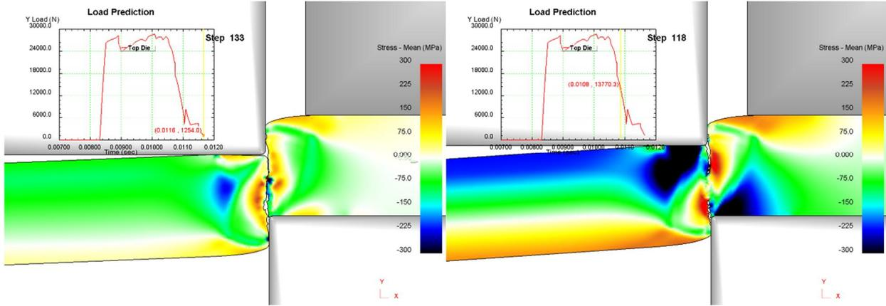
Figure 7: Simulated piercing after the fracture and during the middle of the fracturing process.
