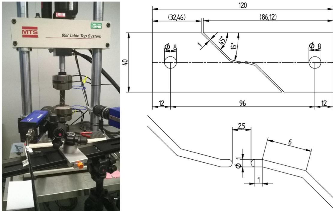
Figure 2: MTS 858 tensile testing equipment setup with the LaVision DIC cameras for shear strain measurement and shear test specimen modified according to recommendations by Tarigopula et al.
