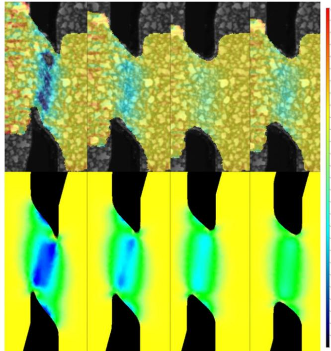
Figure 5: X-Y strains from DIC measurements and simulations at 140, 100, 80 and 60 seconds (the strain colorscale goes from red (0.4) to black (-1) at 0.05 intervals).
