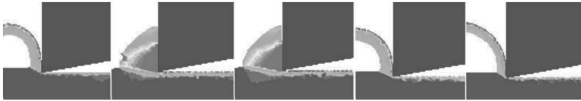
Figure 2. Simulated Plastic Strains. B3 Cutting Conditions, JC1 to JC5 from left to right
