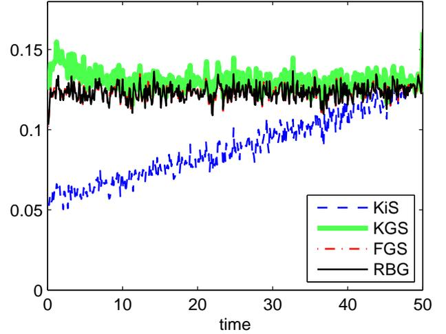
Fig. 3. Predicted error rates with 100 particles averaged over 1000 runs.
