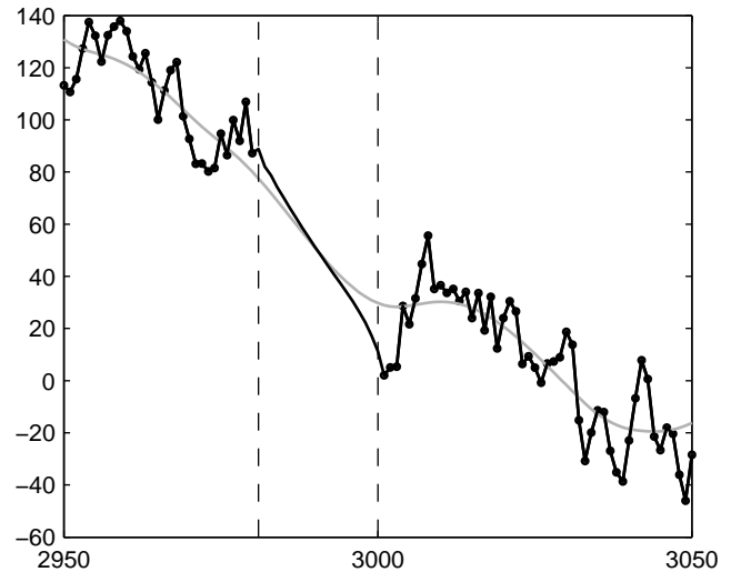
Fig. 6. Prediction over missing data at 2981 – 3000. The gray line is the long term prediction result and black line is the combined long and short term prediction result.
