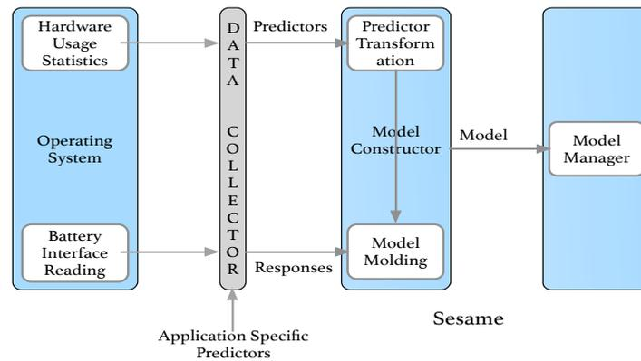
Fig. 8. Sesame architecture for automatic model generation
