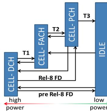
Fig. 5. The HSPA cellular network steps involved in data connectivity.
