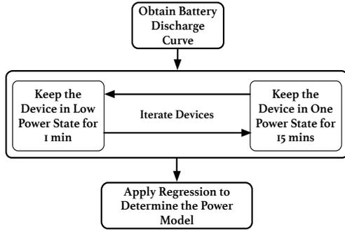
Fig. 6. Overview of the PowerBooter model genera-
