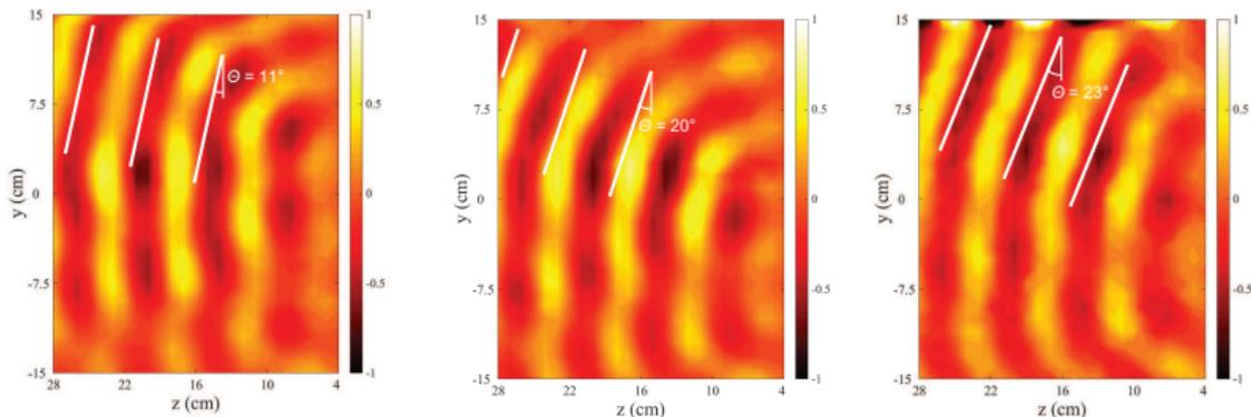
Three primary feeds at different positions create three beams in different directions.
