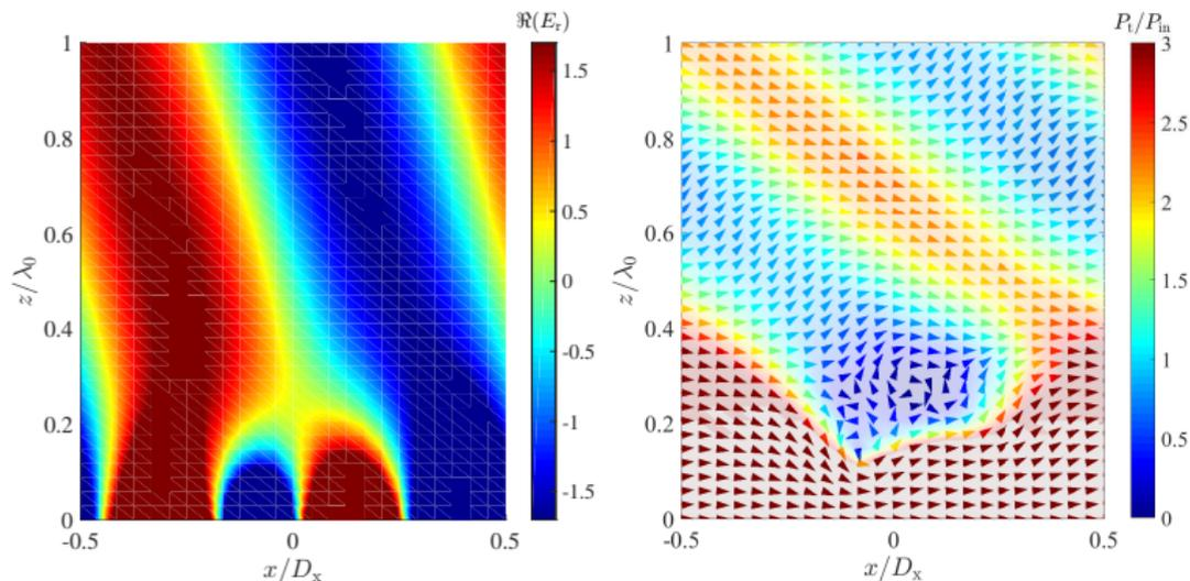
Efficiency 100% with a lossless reflector: an inhomogeneous reactive boundary.
