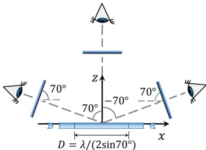
At  $\theta_i = 0^\circ$  and  $\theta_i = \pm 70^\circ$  angles, the observer sees himself as in a mirror normally oriented in respect to him.
