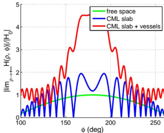
Passive planar reflectors can increase the radiated field more than 2 times (work in progress, C. Valagiannopoulos et al.)
