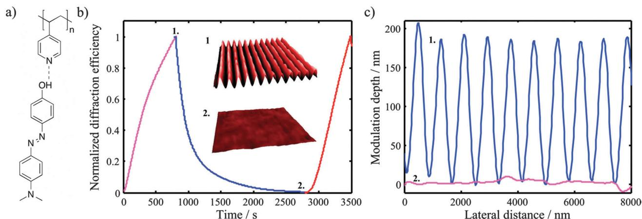
**Fig. 1** (a) The chemical structure of the hydrogen-bonded P4VP–azobenzene complex used in this study. (b) Normalized first-order diffraction efficiency of the SRG inscription (magenta), erasure (blue) and rewriting (red) for the lowest molecular weight complex (1000 g mol<sup>-1</sup>). The inset shows 3D AFM images of the inscribed SRG (1) and the film surface after SRG erasure (2). (c) AFM surface profiles before (1) and after (2) the optical erasure.
