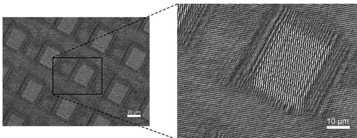
Fig. 3 Scanning electron microscopy images of surface patterns with spatially varying grating vector directions, created by first optically erasing the SRG in non-masked areas (where masking was accomplished by placing a transmission electron microscope grid onto a previously inscribed SRG) and then inscribing another SRG perpendicular to the original one through the mask.
