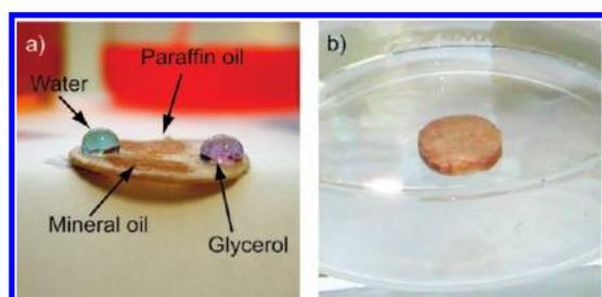
**Figure 2.** (a)  $\text{TiO}_2$ -coated aerogels are hydrophobic and oleophilic: the water and glycerol stay as droplets (colored with Reactive Blue dye for clarity), whereas paraffin oil and mineral oil are readily absorbed. (b) Coated aerogel floating on water (see the Supporting Information, Video S1).
