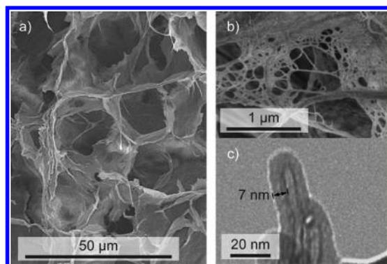
**Figure 1.** Microscopic structure of the native nanocellulose aerogels. SEM micrographs of (a) freeze-dried nanocellulose aerogels with fibrils packed into sheets, which are connected to form an open, porous aerogel structure, and (b) a magnification of a sheet, which is composed of fibrils making the structure also nanoporous. (c) TEM micrograph of a nanocellulose fibril with a uniform 7 nm  $\text{TiO}_2$  coating.
