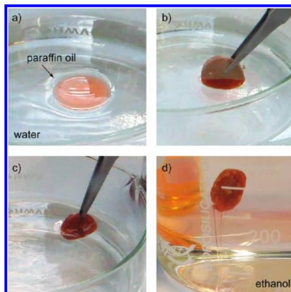
**Figure 3.** Oil spill removal from water (see the Supporting Information, Videos S2 and S3). (a) Paraffin oil (colored for clarity) floating on water; (b) the oil being absorbed into the aerogel; and (c) all of the floating oil has been absorbed. (d) The oil-filled aerogel can be washed simply by immersing it in a solvent, such as ethanol. The oil gets removed as shown by the red streaks.
