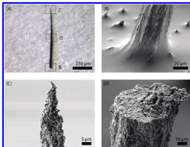
**FIGURE 4.** (A) Optical micrograph of a typical single magnetic cilium with an aspect ratio of 28. Marked areas (B–D) are shown magnified in the scanning electron microscopic images: (B) the cilium base; (C) the cilium tip; (D) the cilium cross section.
