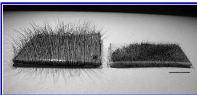
**FIGURE 3.** Photograph of two PTFE substrates covered with magnetic cilia mimics made in a magnetic field of 450 mT with a vertical gradient of 0.1 T/m using the electromagnet (left) and with a vertical gradient of 20 T/m using the permanent magnet (right). The scale bar is 5 mm.
