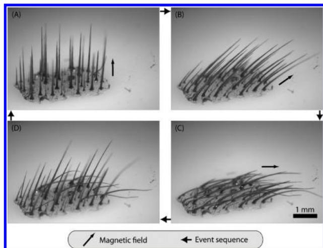
**FIGURE 5.** Magnetic-field-induced bending of the cilia mimics made in a 450 mT magnetic field with a 20 T/m vertical gradient. The magnetic field is (A) perpendicular, (B) at a 45° angle, and (C) parallel to the substrate surface. (D) After removal of the magnetic field, the cilia mimics relaxed toward the surface normally. By reapplication of the perpendicular field, the cilia mimics erected completely once again.
