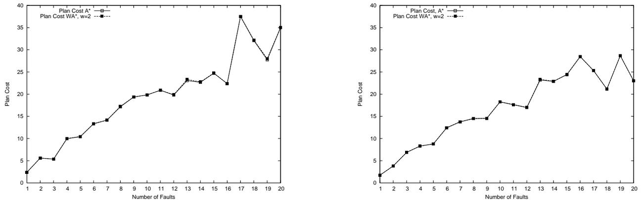
Fig. 7. Average plan cost for the small network (left) and the large network (right).
