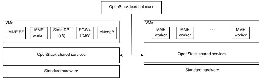
Fig. 2. Overview of the testbed
