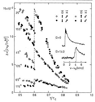
FIG. 2. The frequency shift of the NMR absorption peak in a tilted magnetic field, measured at  $\Omega=1.40$  rad/s. The angle  $\mu$  between  $\Omega$  and H is quoted. The open and filled symbols represent forward and reverse rotation, repsectively. For  $\mu=25^\circ$  and  $155^\circ$ , the directions of  $\Omega$  and H are shown by the arrows. The NMR signals in the inset were measured at  $T/T_c=0.53$  with  $\mu=25^\circ$ .
