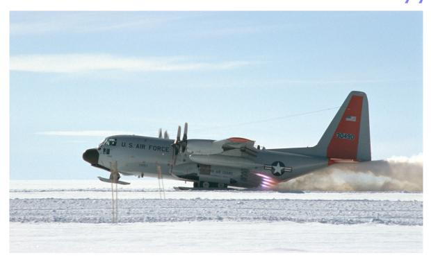
Figure 12.1. A Lockheed Hercules C-130<sup>a</sup> taking off — on skis! — from the NorthGRIP ice-coring site, Greenland, three kilometres above sea level. Note the JATO (jet-assisted take-off) bottles helping out on a runway that is also three kilometres long. Nielsen (2005).
