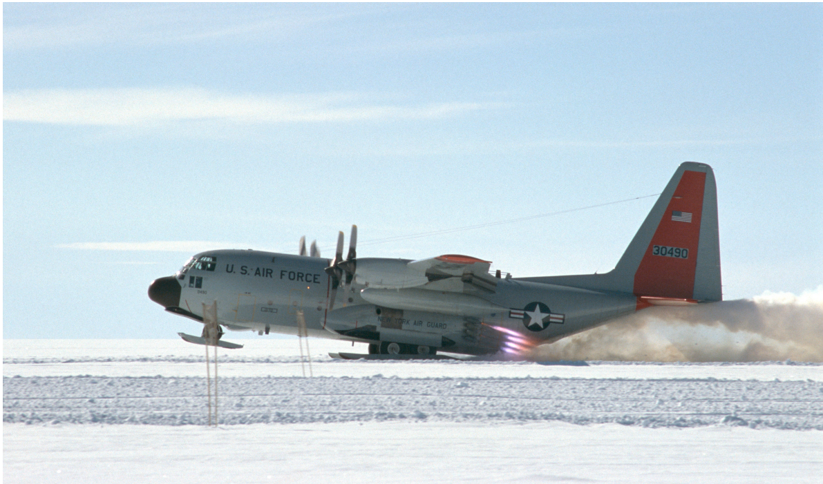
FIGURE 12.1. A Lockheed Hercules C-130 a taking off — on skis! — from the NorthGRIP ice-coring site, Greenland, three kilometres above sea level. Note the JATO (jet-assisted take-off) bottles helping out on a runway that is also three kilometres long. Nielsen (2005).
