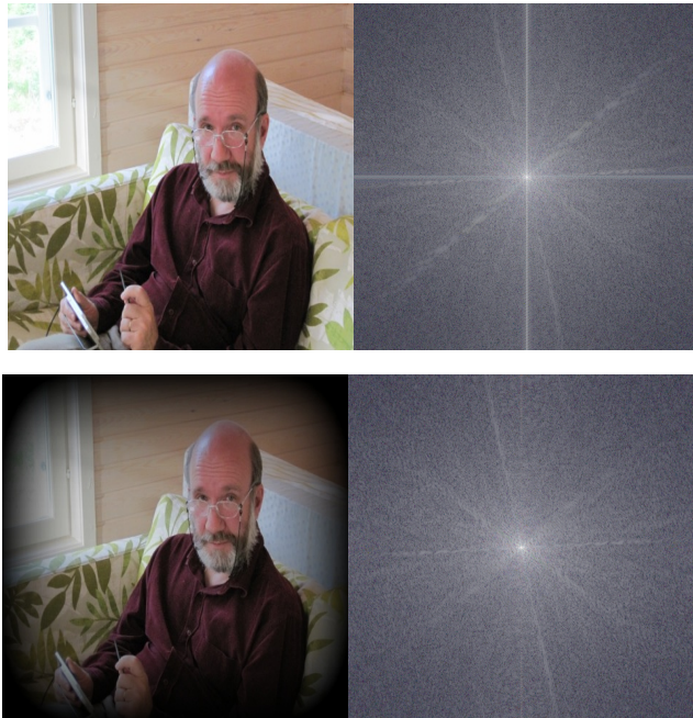
Figure 9.4. Example images for FFT transform without (above) and with (below) tapering. Used on-line FFT service Watts (2004).
