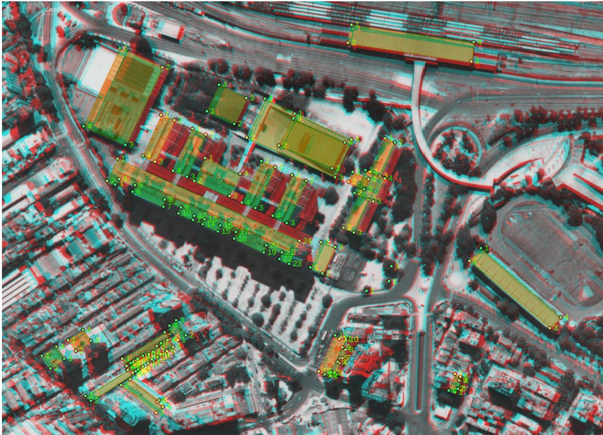
FIGURE 10.9. A bigger sample of stereo plotter production showing several urban features in the Rio area.
