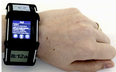
Figure 8. Facet is a multi-display bracelet consisting of independent touch-sensitive segments.
