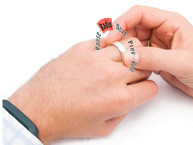
Figure 7. Nenya is a magnetic ring allowing simple input actions such as twist to select and slide to click.
