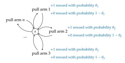
Figure 15.1. The multiarmed bandit problem is a single-state MDP where actions can differ only in the likelihood that they produce reward.
