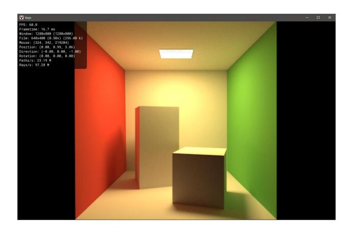
Improvement of the path tracing implementation in Valo. The previous version used the megakernel approach, which was not very performant. The wavefront method improved performance, but not that significantly, as GPUs have become better at handling megakernel type of workloads.
