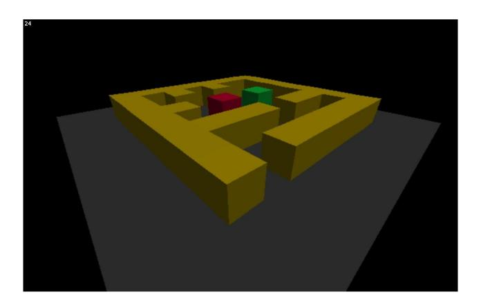
Pymazing is a basic 3D software rasterizer that does all the drawing/rasterization and 3D math in pure Python and Numpy. Levels ("mazes") can be loaded from image files in which each pixel represents a colored cube in the 3D world.
