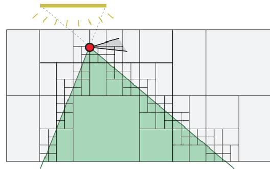
**Figure 4:** A 2D cross-section illustrating the “rasterization” of a wedge into a hierarchical grid. The data structure used for determining the regions occupied by a given wedge is an axis-aligned BSP tree, whose nodes keep track of wedges that either intersect or fully contain the node.
