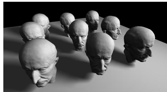
**Figure 1:** Physically-based soft shadows in a 900k triangle scene. Here the previous soft shadow volume method of Laine et al. [LAA\*05] is slower than the reference ray tracer, while we achieve a speedup factor of 12.3 over the previous method and a factor of 6.8 over the reference ray tracer.
