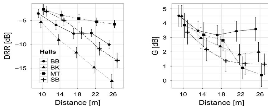
Figure 2 DRR and G averages over source positions and 500 Hz and 1 kHz centered octave frequency bands. Bars represent the 95 % confidence intervals, calculated from the variation over 24 source positions and the two frequency bands and give an indication of how much the position on the stage influences the value of the parameter.
