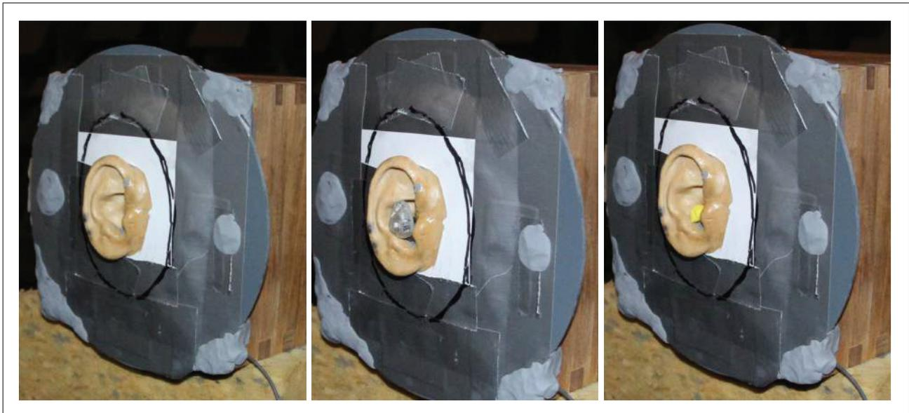
Figure 3. The measured earplugs. From left: open ear canal, active earplug, and standard EAR.
