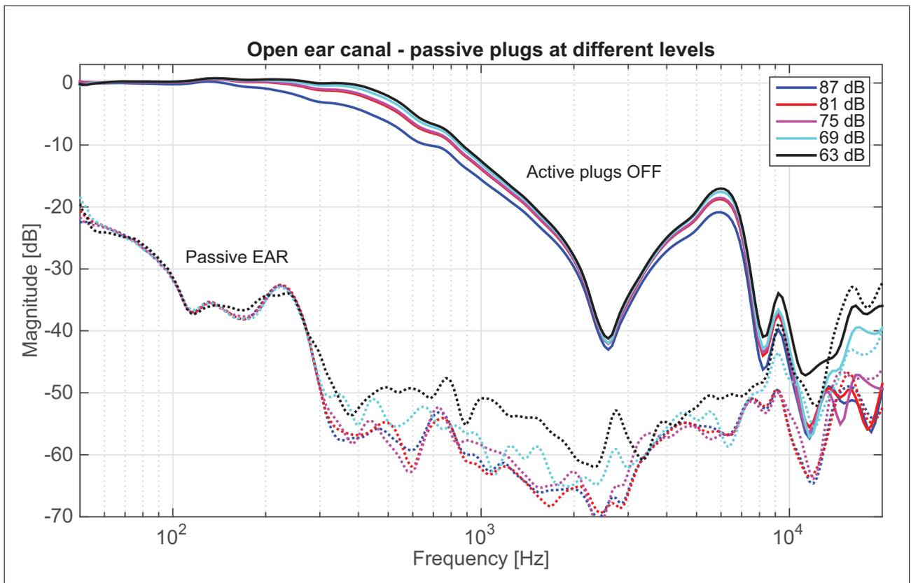
Figure 6. Frequency responses (1/3 octave smoothed) of the difference between open ear canal and passive earplugs.
