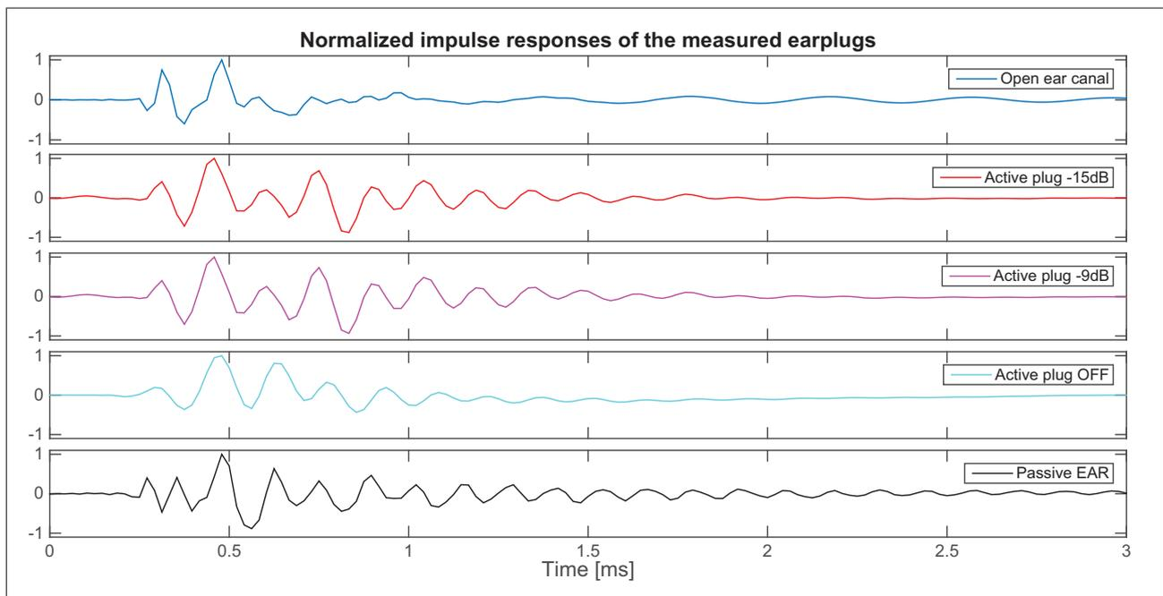
Figure 4. Early part of the measured impulse responses at  $L_{AS} = 87$  dB.
