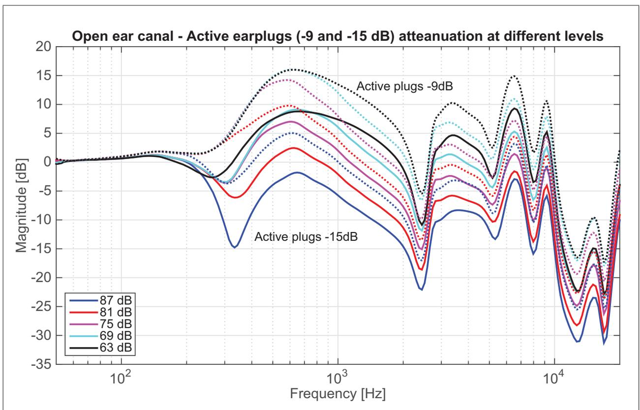
Figure 7. Frequency responses (1/3 octave smoothed) of the difference between open ear canal and active earplugs.
