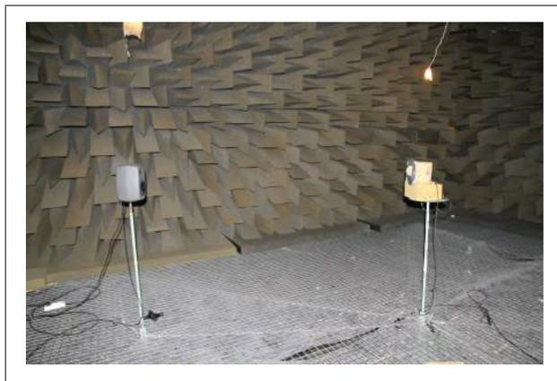
Figure 1. The measurement setup in an anechoic chamber, the distance between the loudspeaker and the ear simulator is 2m.
