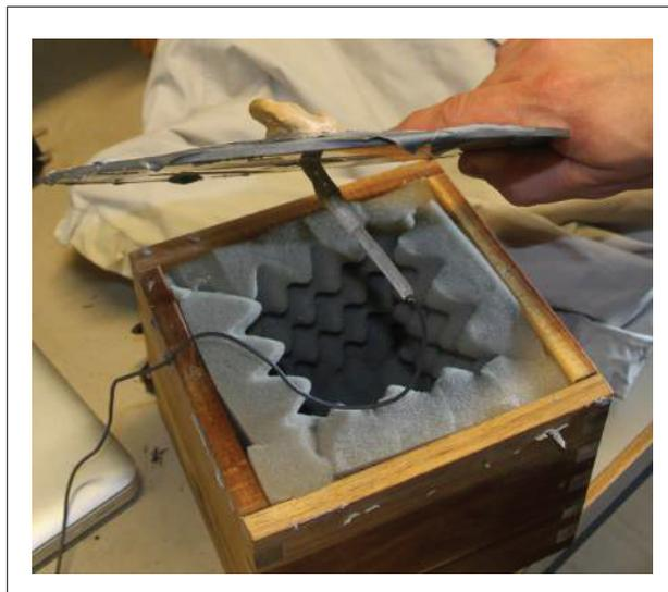
Figure 2. The used ear simulator. The ear canal is made of a plastic tube and the microphone is in the end of this tube at the position of the tympanic membrane.
