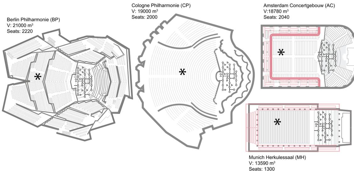
FIG. 3. (Color online) Blueprints of the concert halls. Star indicates the measurement positions at 19 meter distance from the position of the first violin.
