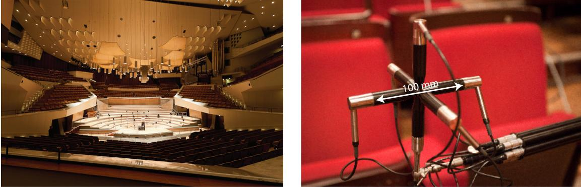
**Figure 1:** The loudspeaker orchestra (left) and the microphone array (right). The results in this paper are obtained with 25 mm microphone spacing instead of the shown 100 mm spacing.
