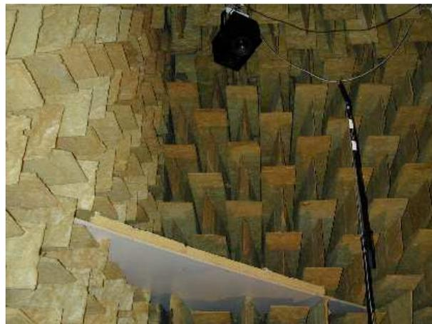
Figure 1: *The measurement setup. In reported results, the microphone was positioned under the chipboard plate.*
