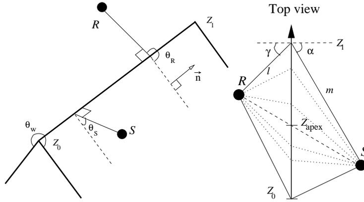
Figure 2: Geometry of a finite wedge. On the right sound paths via edge points  $Z_0$  and  $Z_1$  are indicated by the solid lines, the least-time sound path via the apex point  $Z_{\text{apex}}$  is depicted with dashed line and some other sound paths are illustrated with dotted lines.
