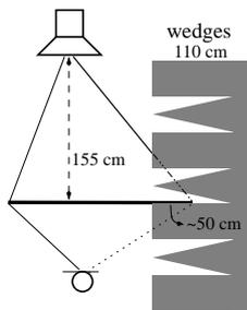
Figure 5: The schematic drawing of the setup for measuring diffraction from a single edge. Diffraction from the edge between the mineral wool wedges is attenuated since the sound has to travel through several absorptive wedges.
