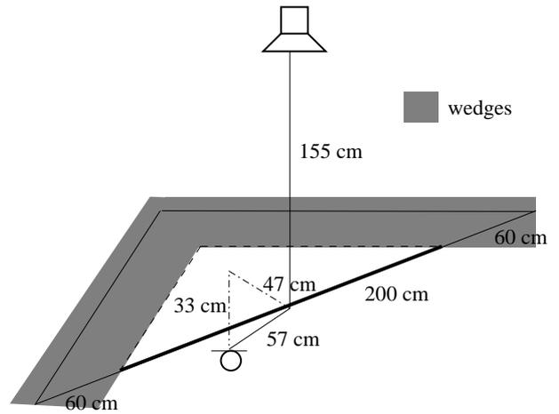
Figure 3: The positions of the loudspeaker and the measurement microphone. Note that board occludes the sound source in the measurement position.
