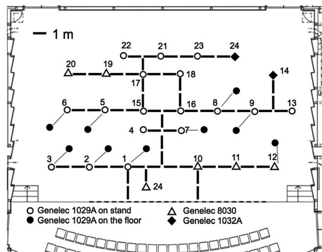
FIG. 3. Layout of the loudspeaker orchestra on the stage of a concert hall.
