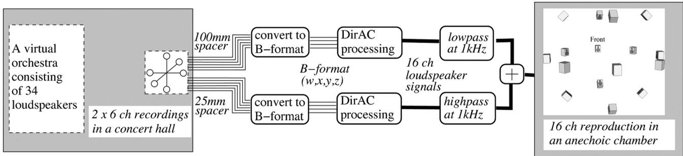
FIG. 2. Signal processing chain to obtain comparable stimuli for the subjective evaluation. The loudspeaker orchestra is recorded with 6 microphones twice, with 25 mm spacer and 100 mm spacer. Both six microphone signals are converted to B-format signals that are processed with DirAC for rendering sound with 16 loudspeakers in an anechoic chamber.
