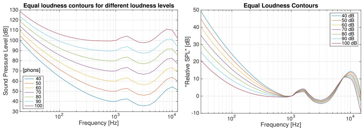
**Figure 4: Left: Equal loudness contours according to ISO226 standard. Right: The same contours level aligned at 1 kHz.**
