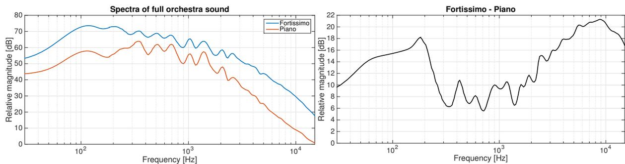
**Figure 2: Left: The spectra of a full orchestra sound in different dynamics. Right: the spectral change between *fortissimo* and *piano*.**
