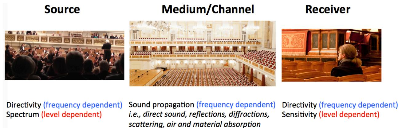
**Figure 1: Source - Medium - Receiver communication process for a concert hall.**
