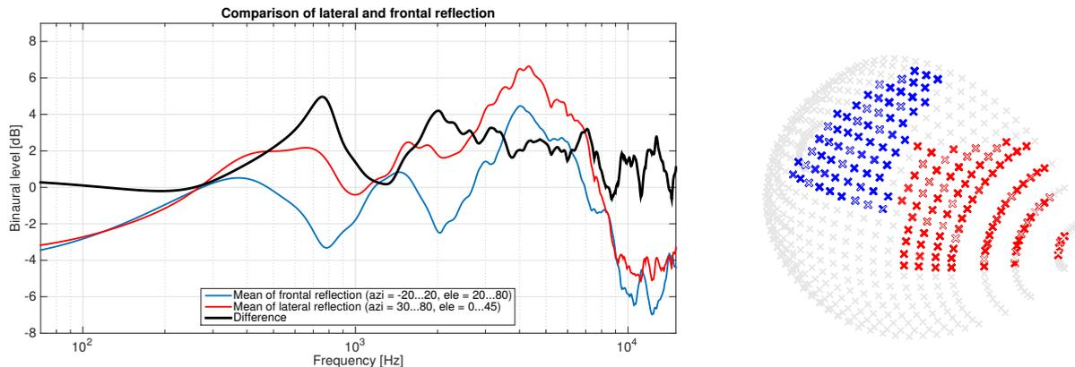
**Figure 3: Left: Binaural level for reflections from lateral and frontal directions. The responses are means of all colored directions illustrated on the right.**
