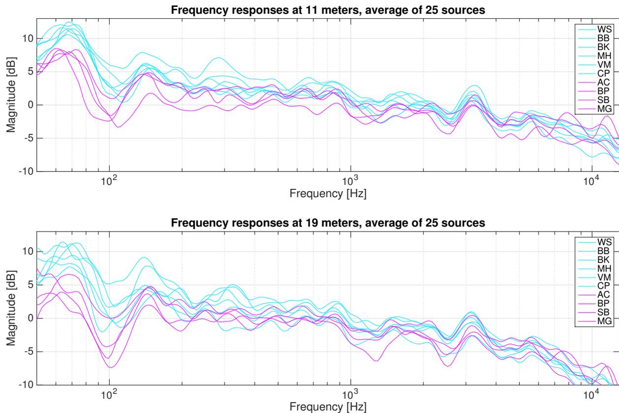
Figure 4: Frequency responses of 10 different concert halls, measured with the loud-speaker orchestra in two different receiver positions.
