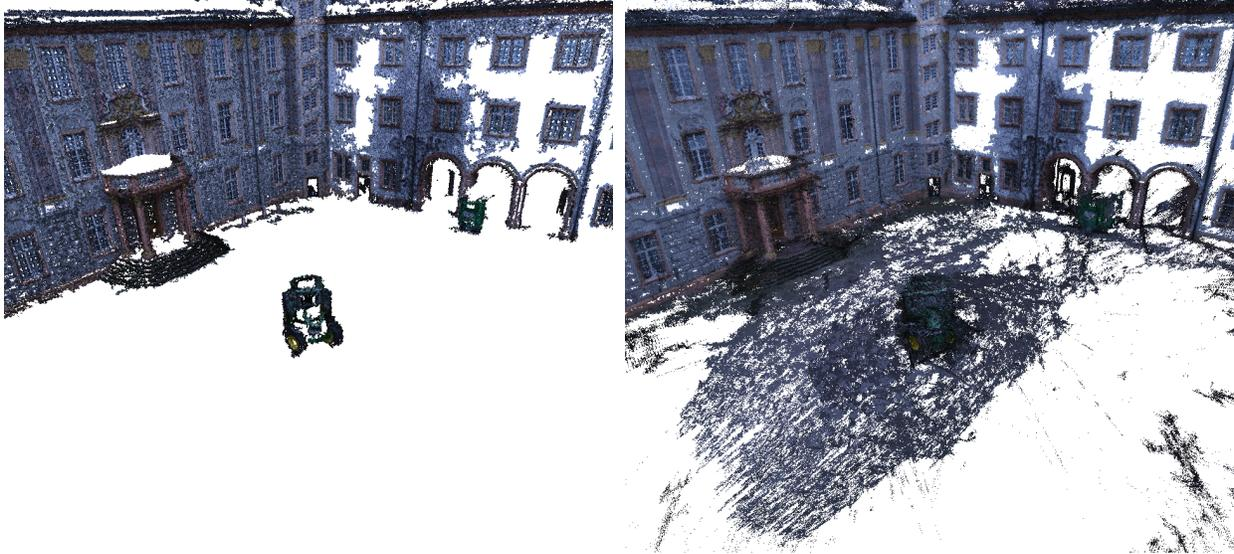
Figure 11. Castle reconstructions build by the PMVS program [3] (left) and the proposed method (right). Our reconstruction has lots of points on ground which is totally missing in the PMVS reconstruction.
