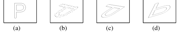
Fig. 1: Pattern matching: original (a), transformed and noise added (b), recovered transformation with MSAP (c), and with MD (d).
