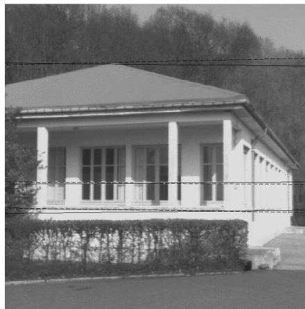
Figure 11: The second image and epipolar lines. Solid line from Bayes-estimate, dashed from calibrated F-matrix.
