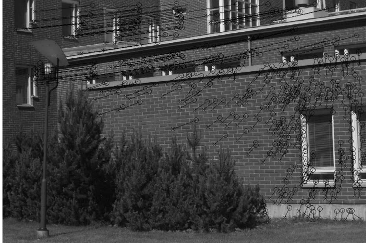
Figure 4: Matched points from the second (x) and the first (o) image plotted in the second image. Points are obtained by ImageMatching-software.
