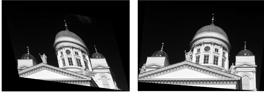
Figure 7: Rectified image pair. The rectifying transformation for the first image is obtained by minimizing the disparity between rectified images.
