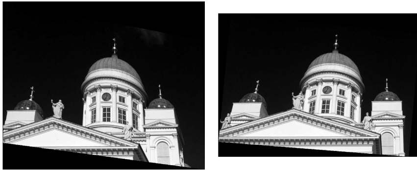
Figure 8: Rectified image pair. The rectifying transformation for the first image is obtained by minimizing the disparity between the original and rectified image.
