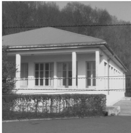
Figure 10: The second image and epipolar lines. Solid line from LMedS-estimate, dashed from calibrated F-matrix.
