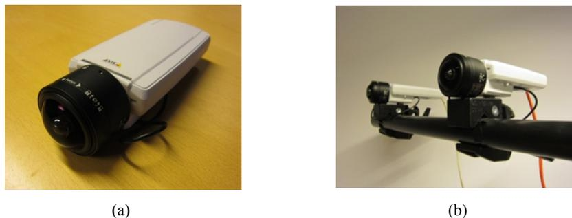
Figure 2. (a) Panomorph Lens YF360A-SA2 and Network Camera AXIS P1346-E. (b) The flexible spherical stereoscopic vision system.
