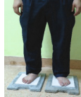
Fig. 2. The inability to distinguish between correctly and incorrectly laid tiles by standing on them
