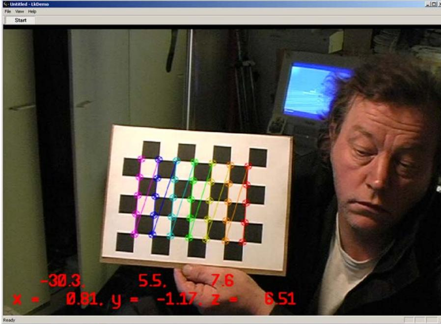
Figure 2: Used checkerboard pattern in Zhang camera calibration implementation. Red numbers in the bottom area of the picture describes rotation and translation of checkerboard.
