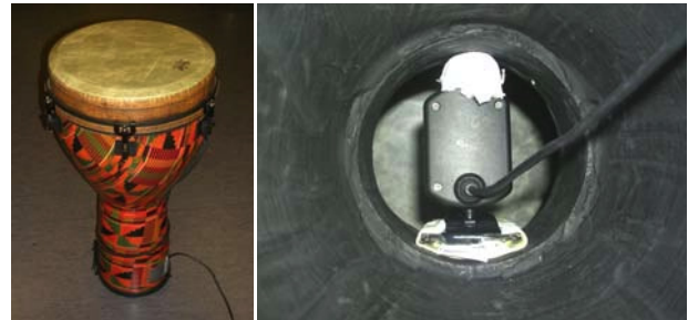
Figure 3. A web camera is mounted inside the physical djembe, facing towards the membrane. The software runs on a Windows laptop. Good speakers are also needed as the sound contains mostly low frequencies.
