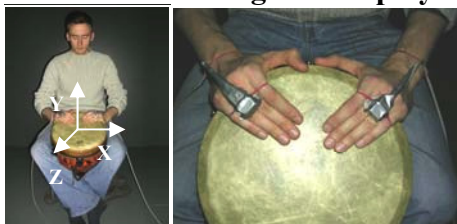
Figure 1. Recording setup for analyzing hand motion during real-life djembe playing. To record hand motion, a magnetic motion sensor is attached to each hand.
