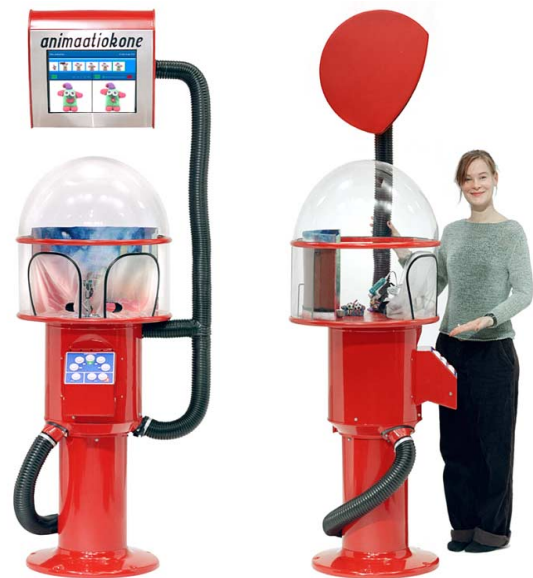
Figure 1. Front and side views of Animaatiokone. Animating takes place inside the transparent studio dome. The user interface consists of a camera and a button panel inside the dome, the computer display and microphone embedded above the dome and second panel in the front.
