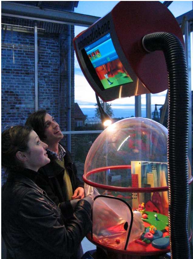
Figure 8. Using Animaatiokone. Animating takes place inside the studio dome, where there's a backdrop and a movable camera. The display above the dome allows people around to watch the animator at work.
