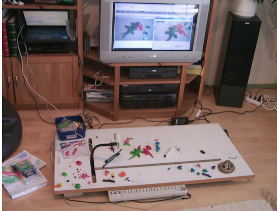
Figure 4. The low-tech installation prototype consisting of a television, a drawing/modeling surface, a rail-mounted camera, and a stripped-down keyboard attached to the front.
