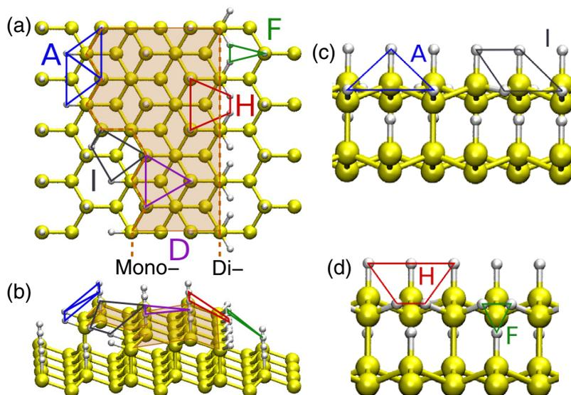
**Figure 5.** Some important Cu adsorption sites with labels introduced in [24]. Examples of sites A, D, F, H and I are shown. In panels (a) and (b), a structure with two (111) layers is shown (upper layer is shaded). The left side of the layer is a kinked monohydride step and the right side a dihydride step. Panels (c) and (d) show side views of the monohydride and dihydride steps, respectively.
