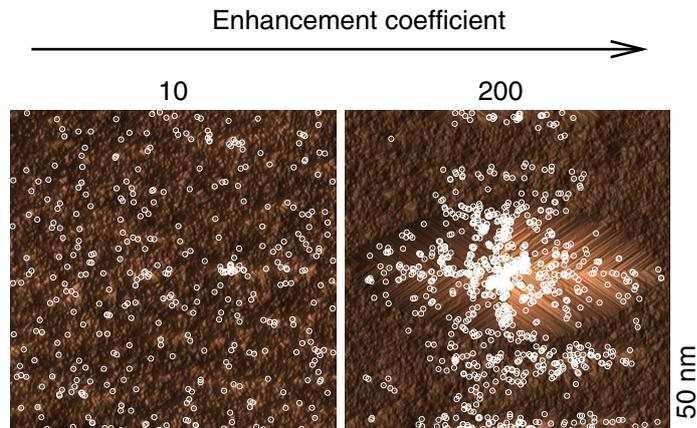
**Figure 8.** Surfaces ( $150 \times 150 \text{ nm}^2$ ) simulated under HEA with 1100 Cu atoms after 50 million Si removals. Adsorbed Cu are shown as circles (size exaggerated). The enhancement coefficient ( $a$  in (3)) is varied as shown.
