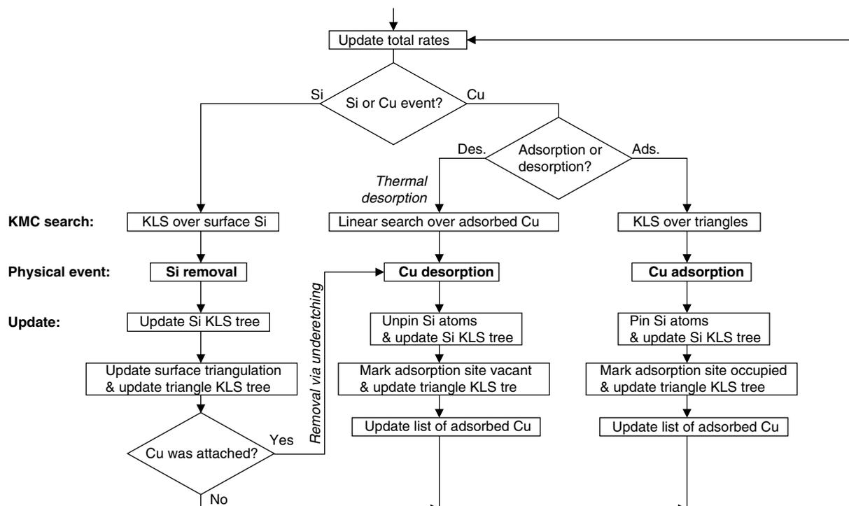
**Figure A.1.** Flowchart presentation of the used hybrid search tree. The choices between Si and Cu events are made stochastically according to the relative probabilities of the events. If we remove a Si atom to which a Cu is connected, the Cu desorbs automatically due to underetching.
