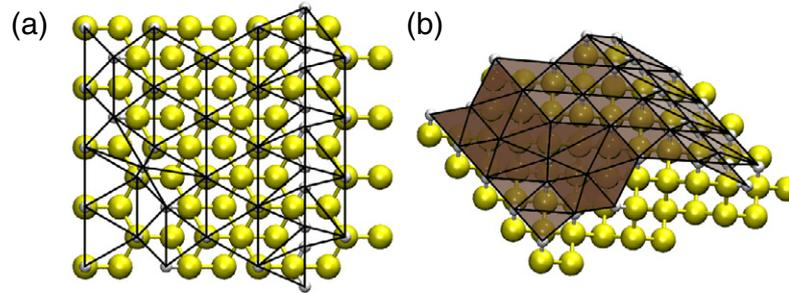
**Figure 1.** An example of the surface triangulation from (a) a top-down and (b) an isometric perspective (latter with shading). Small spheres located at the triangle vertices are hydrogen. The larger spheres are silicon.
