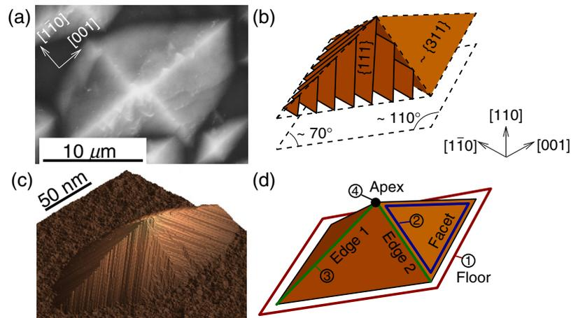
**Figure 4.** The experimentally observed trapezoidal hillocks on Si(110) [11] in (a) should ideally consist of stacks of triangular (111) layers [17], as in (b). This hypothetical structure is realized in the simulations, as in (c) (using IEA). (d) Lists the parts of a hillock whose relative stability determines how the structure evolves: (1) floor, (2) facets, (3) facet edges and (4) apex.
