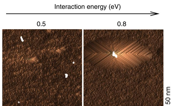
**Figure 7.** Surfaces ( $150 \times 150 \text{ nm}^2$ ) simulated under IEA with 115 Cu atoms after 50 million Si removals. Adsorbed Cu are shown as circles (size exaggerated). The enhancing factor  $f^{\text{IEA}} = \exp(E/k_{\text{B}}T)$  is varied via the interaction energy  $E$ , as shown.
