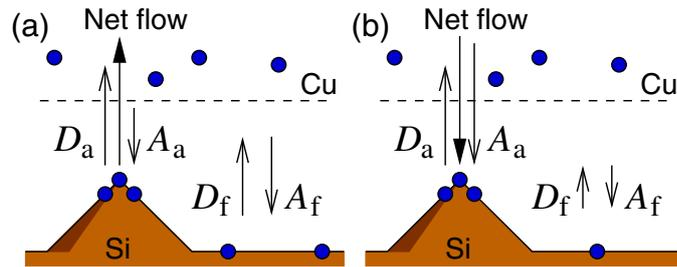
**Figure 2.** The conditions resulting from a morphological fluctuation for (a) uniform and (b) NUA. The arrows represent the flux of Cu atoms: adsorption ( $A$ ) and desorption ( $D$ ) at the apex (a) and on the floor (f).
