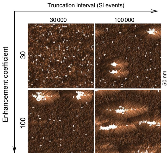
**Figure 9.** Surfaces ( $150 \times 150 \text{ nm}^2$ ) simulated under AEA with 450 Cu atoms after 50 million Si removals. Adsorbed Cu are shown as circles (size exaggerated). The interval between activity truncations and the enhancement coefficient ( $b$  in (5)) are varied as shown.
