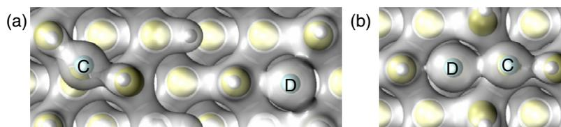
**Figure 3.** Electron densities plotted at an isosurface of  $0.019 \text{ e \AA}^{-3}$  around two Cu atoms when they are (a) apart or (b) next to each other on the H-terminated Si surface. In both cases the Cu are at (111) terrace sites C and D.
