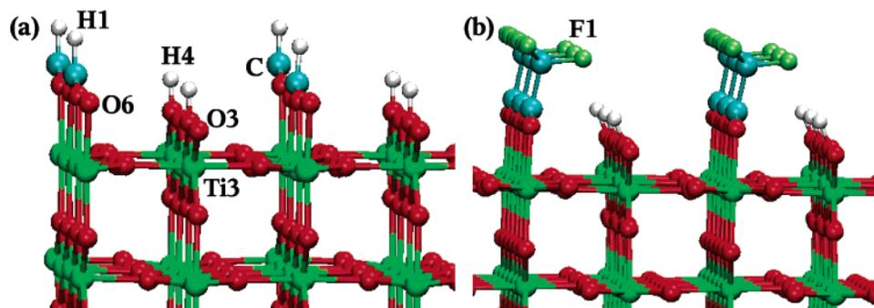
**Figure 1.** Calculated structures of monolayers of (a) formate and (b) trifluoroacetate adsorbed on the TiO<sub>2</sub>(110) surface with key sites labeled.
