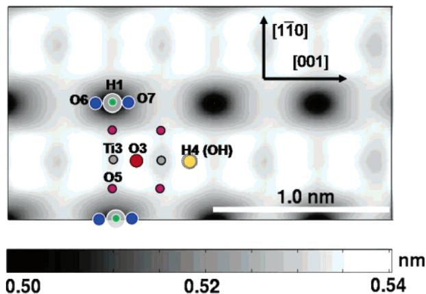
**Figure 5.** Modeled NC-AFM image of formate monolayer on the TiO<sub>2</sub>(110) surface. The tip radius is 50 nm, the normalized frequency shift is 3.5 fN m<sup>1/2</sup>, the cantilever stiffness is 35 N/m, and the peak-to-peak oscillation amplitude is 10 nm. Colored circles draw correspondence between atomic sites and areas of the image. Red, magenta, yellow, and blue circles represent, correspondingly, bridging, surface, hydroxyl, and formate oxygen atoms.
