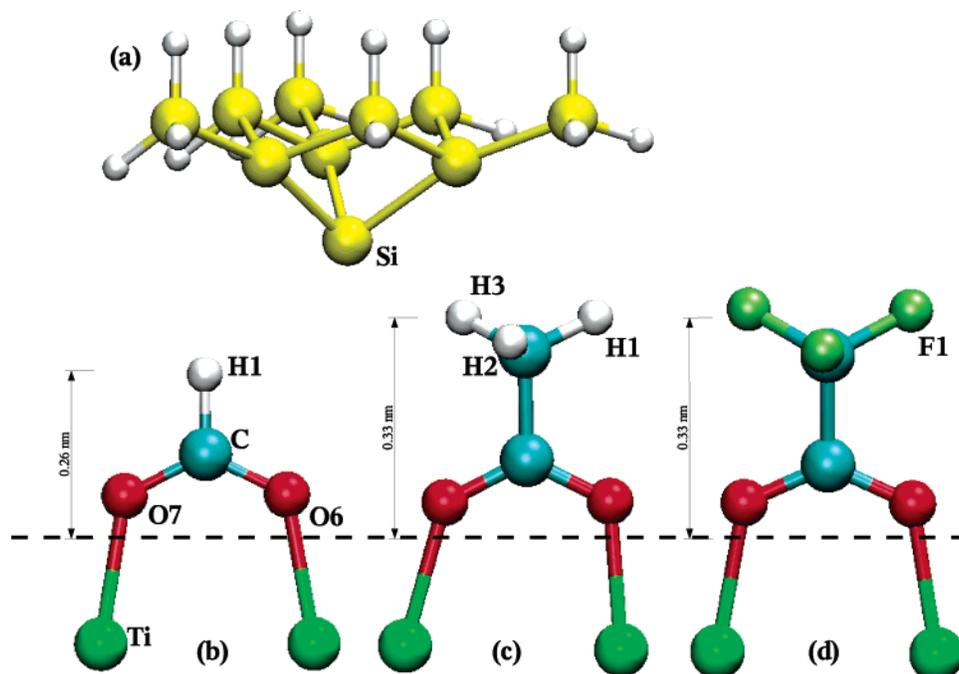
**Figure 2.** Schematic figure showing the structure of (a) the silicon tip and the adsorbed structure of the (b) formate, (c) acetate, and (d) 3F-acetate molecules on the TiO<sub>2</sub>(110) surface. The dashed line shows the height of the bridging oxygen row as a reference for the heights of the molecules.
