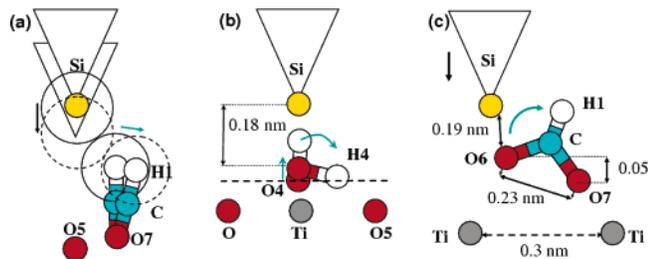
**Figure 4.** Schematic representation of displacements induced in the TiO<sub>2</sub> surface and adsorbed formate monolayer by the Si tip with dangling bond approaching (a) an O5 site next to the formate molecule; (b) a hydroxylated oxygen (H4); and (c) an O7 site next to the formate molecule. The bold dashed line indicates the level of bridging oxygen atoms as the reference for the height of the molecule.
