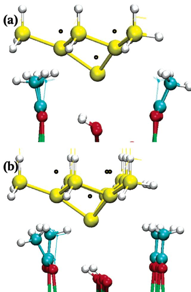
**Figure 7.** Displacements of atoms as the tip approaches over the acetate monolayer at sites (a) Ti3 and (b) H4. The positions at larger tip-surface distance are shown by dots and lines, whereas the closest approach is shown by atoms and bonds. The distances are 0.1 and 0.05 nm in part a and 0.2 and 0.05 nm in part b.
