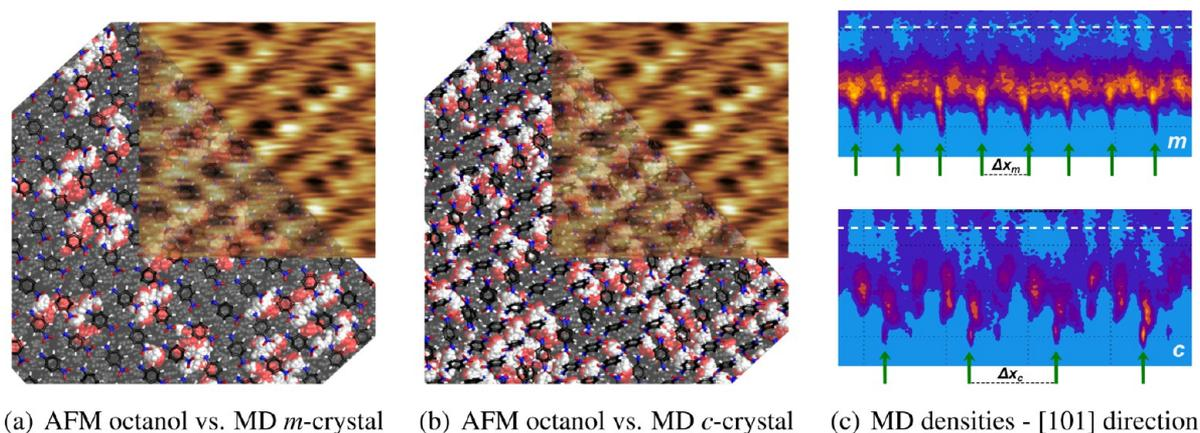
**Figure 5.** Composite images comparing the AFM octanol topography images to both the MD snapshots for the *m*-crystal (a) and the *c*-crystal (b). In panel c, the cross-sectional density plots along the [101] direction as obtained from the MD simulations are shown, with the periodicity indicated by the green arrows.
