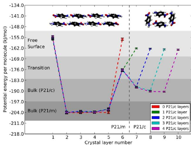
**Figure 6.** Potential energy per molecule in each layer of a combined *m*-crystal and *c* crystal *p*-nitroaniline structure. The different curves show the effects of none, one, or more *c*-crystal layers on top of a bulk *m*-crystal structure. The outer layers are exposed to vacuum, hence the free layers. The molecular arrangement is shown on top. (See also Figure 1d.)
