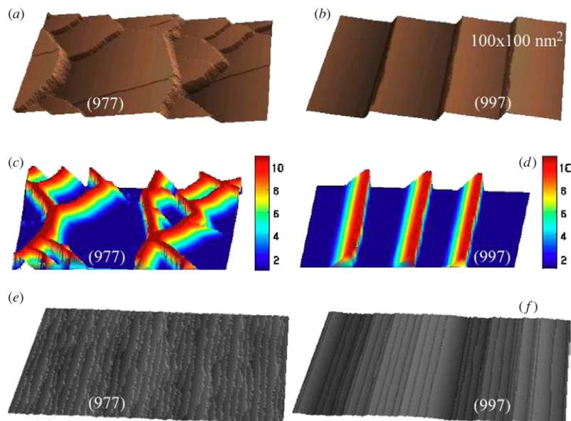
**Figure 18.** Examples of simulated  $(h h h \pm 2)$  surfaces: (a)–(b) morphologies showing bunching; (c)–(d) diffusion factor for (a) and (b) showing the existence of inhomogeneities; (e)–(f) morphologies without diffusion inhomogeneities. Step bunching in (a) through (d) generated using the IAM method ( $a = 10.0$ ,  $\Delta T = 0.4$ ,  $A_{\max} = 18$ ,  $\Delta A = 1$ ). No bunching in (e) and (f) obtained with  $a = 0$ . step-flow parameters as in column 2 of table 1 (low concentration).
