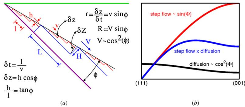
Figure 35. (a) Etch rate for a simple step-flow model with (R) and without (r) step bunching. (b) Effect of step bunching on the etch rate.
