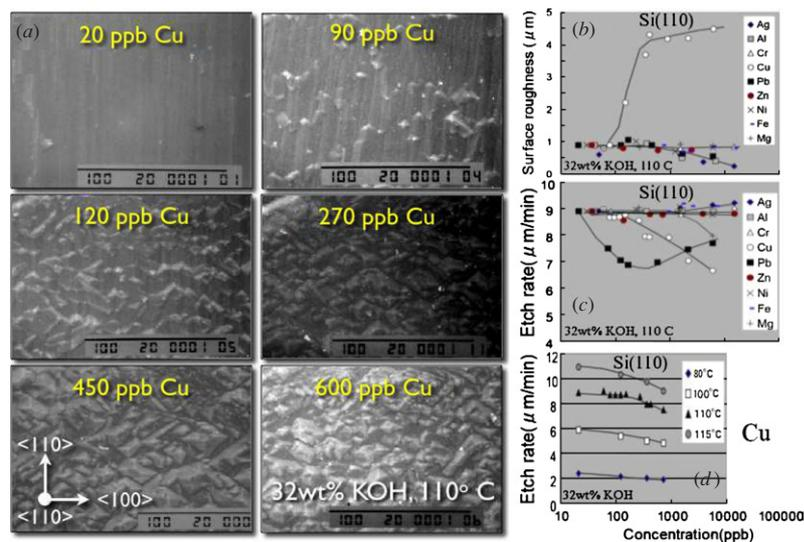
**Figure 31.** Effect of the addition of metal impurities on (a) the morphology, (b) the surface roughness and (c), (d) the etch rate of Si(110). From [72] (pp 36, 38, 39, 44).
