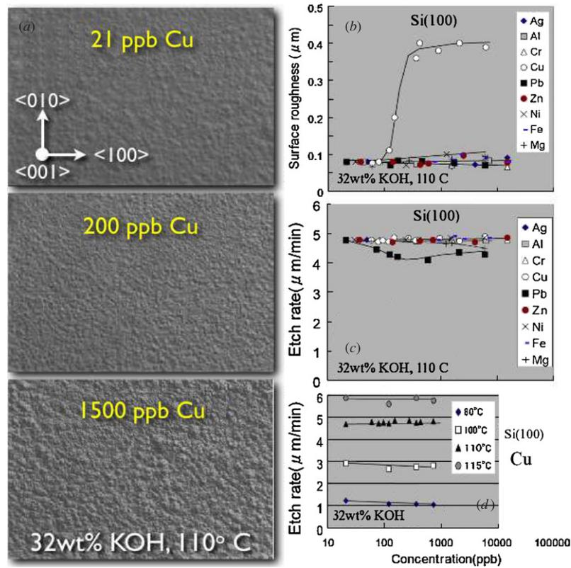
**Figure 32.** Effect of the addition of metal impurities on (a) the morphology, (b) the surface roughness and (c), (d) the etch rate of Si(100). From [72] p 36, 38, 39, 42.
