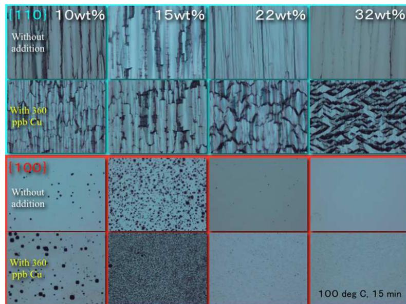
**Figure 33.** Effect of Cu impurities on the surface morphology at different concentrations. Denso Corp. unpublished.
