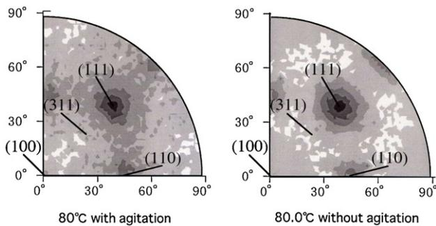
Figure 36. Stereographic projection of the etch rate showing the shift in the etch rate maximum due to stirring in 10 vol% TMAH. Sato Laboratory.
