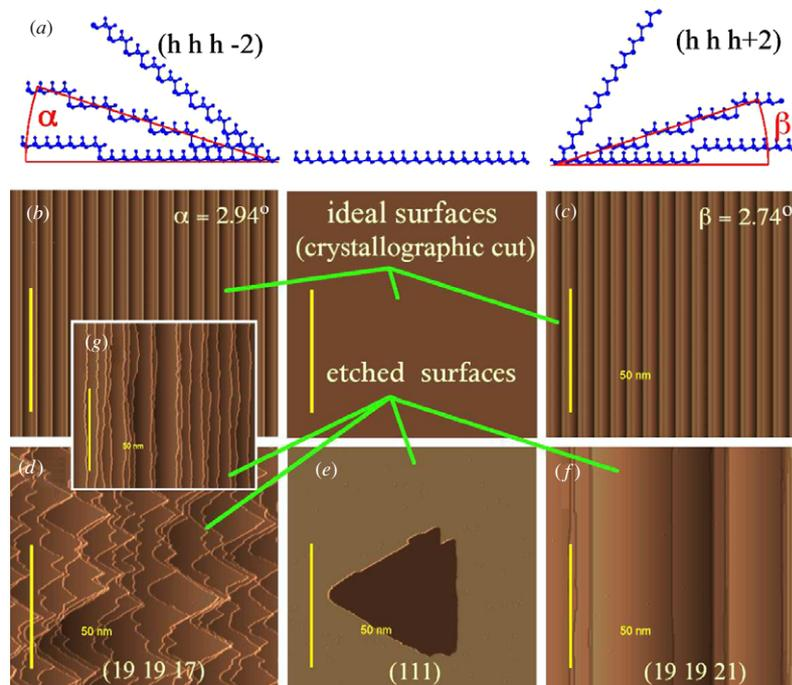
**Figure 14.** Different surface morphologies on miscut (1 1 1) at high concentration. Simulation.
