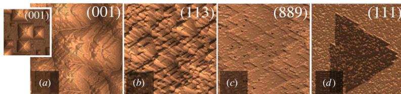
**Figure 24.** Relation between pyramidal hillocks on (1 0 0) and polygonal steps on ( $h h h + 2$ ). (From simulations.) This figure contains frames from figure 14 of [43].
