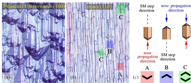
**Figure 22.** Nosed zigzag structures on vicinal and exact (1 1 0). Experimental images (a), (b) from Sato Laboratory, Nagoya University (unpublished).
