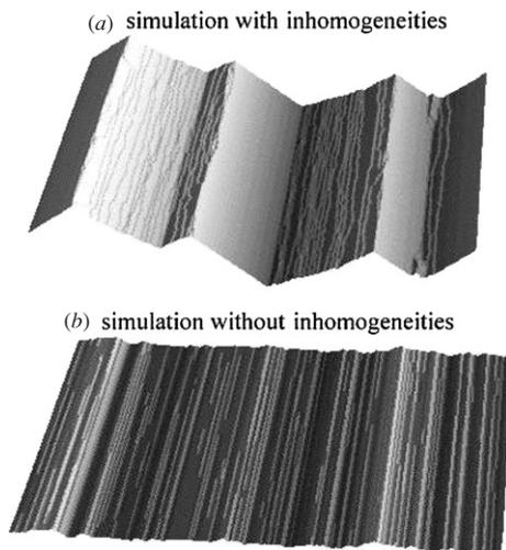
**Figure 21.** Formation of zigzag structures on (1 1 0). (a) Simulation using IAM ( $a = 2.0$ ,  $\Delta T = 1.4$ ,  $A_{\max} = 18$ ,  $\Delta A = 1$ ). (b) Simulation without inhomogeneities ( $a = 0$ ). System size is  $100 \times 100 \text{ nm}^2$ . Compare to figure 19(a). From [29] (figure 12).
