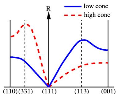
**Figure 38.** Typical variation of the etch rate at low and high concentration.
