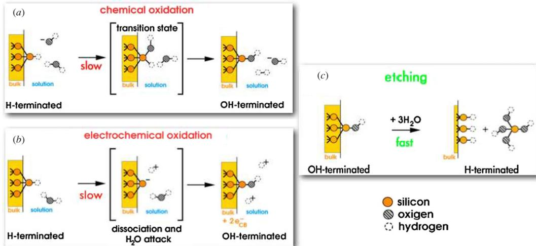
**Figure 3.** Cartoon-like description of the sequential oxidation and etching reactions taking place during etching. Only the nearest underlying bulk atoms in the neighborhood of the surface site are depicted. From [46] (modification of figures 5, 6 and 7).
