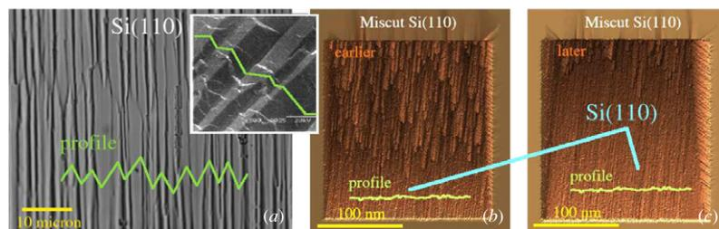
**Figure 19.** (a) Experimental zigzag structures on (1 1 0) (large frame from figure 8 of [42] with permission from Elsevier; small frame from p 125 of [72]). (b), (c) Simulated morphology with a step-flow model that disregards step bunching and micromasking.
