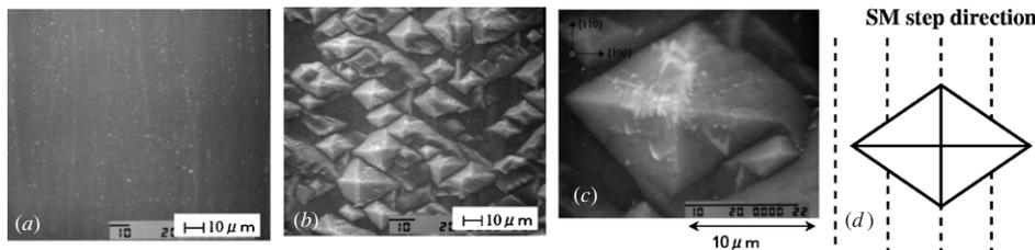
**Figure 29.** (a), (b) Comparison of the (1 1 0) morphology with and without hillocks. (c) Detail of a hillock in (b). 32 wt% KOH, 110 C. (d) Projection of the idealized hillock shape on the floor surface. For (a) Cu content is 21 ppb. For (b) and (c) Cu content is 360 ppb. From [72].
