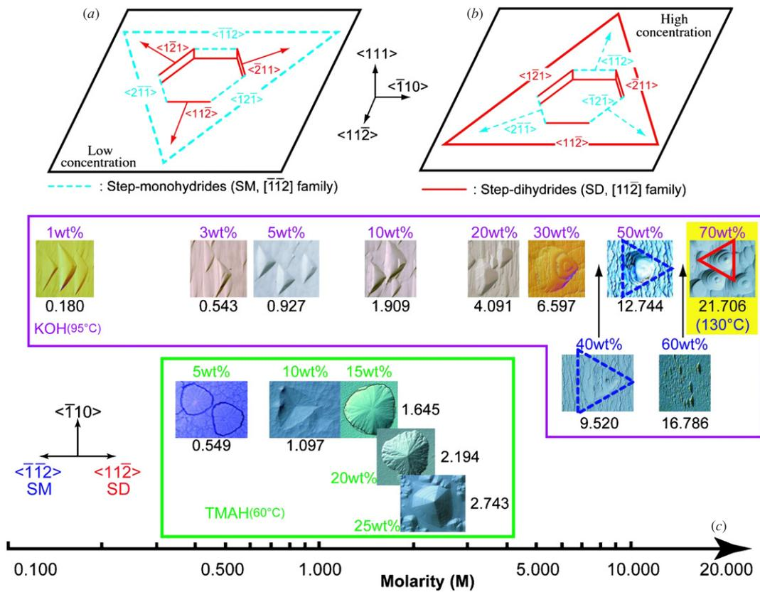
Figure 9. Etch pit shape dependence on etchant concentration. Frame (c) from [66] (figure 3) with permission © 2006 IEEE.
