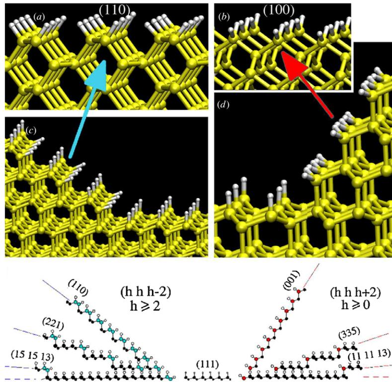
Figure 8. (1 1 0) and (1 0 0) as limiting examples of stepped (1 1 1) surfaces.
