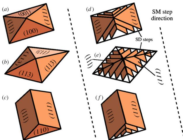
**Figure 30.** (a)–(c) Schematic potential shapes for morphology features on (1 1 0). (d)–(f) Description of the shapes using (1 1 1) terraces.
