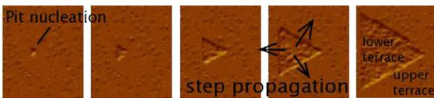
**Figure 4.** Pit nucleation and step propagation on (1 1 1). Simulation.
