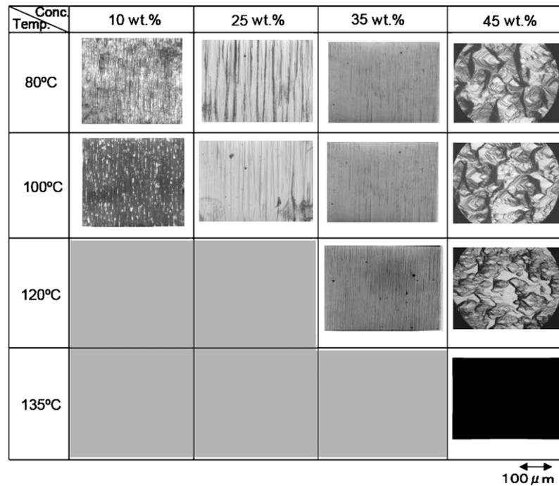
**Figure 28.** Morphology of (1 1 0) as a function of KOH concentration and temperature. From [72] (p 23).
