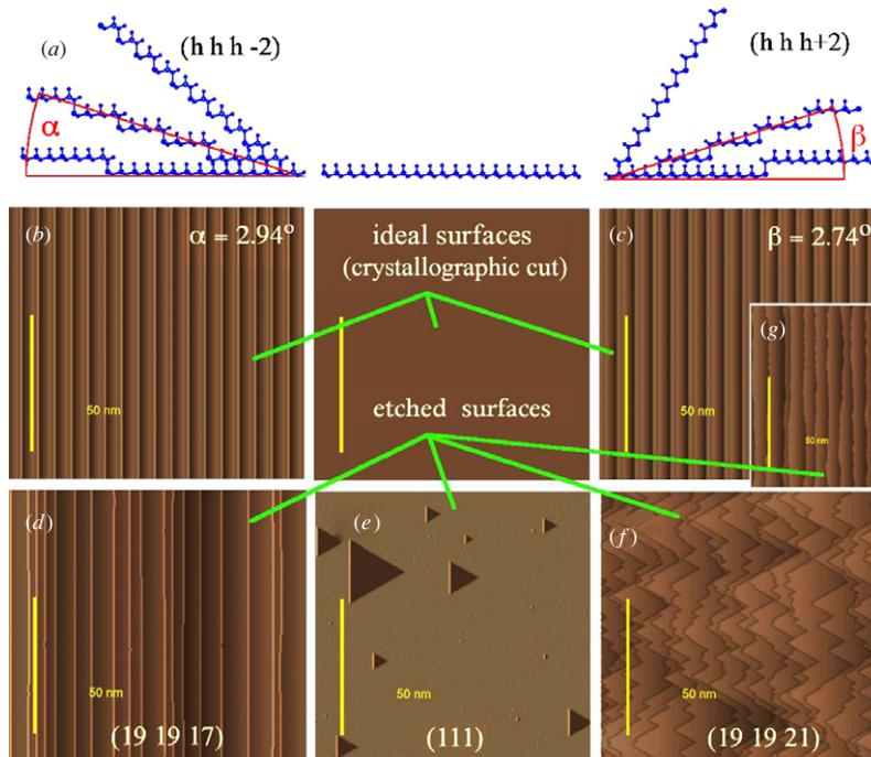
**Figure 12.** Different surface morphologies on miscut (1 1 1) at low concentration. Simulation.
