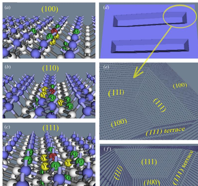
**Figure 2.** Link between microscopic structure and macroscopic anisotropy during etching. (a)–(c) Typical atoms on each principal surface are shown in red color (R) and their first (second) neighbors in yellow (Y) (green (G)); (d) Example of a 3D etched structure on a (1 0 0) wafer (misaligned trenches); (e)–(f) Details of the region highlighted in (d), showing the slow etching (1 1 1) surfaces.
