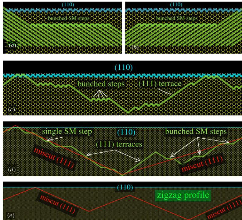
**Figure 20.** Schematic formation of a zigzag profile on (1 1 0) due to step bunching. From [29] (figure 11).
