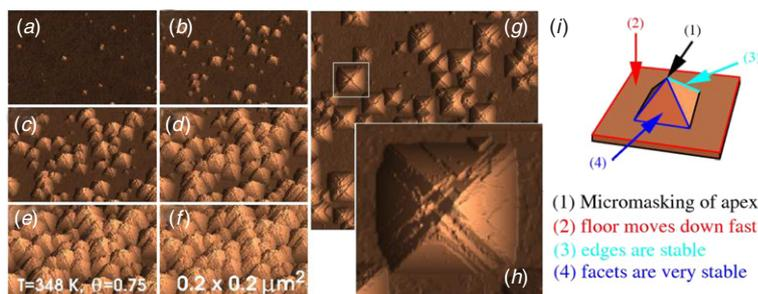
**Figure 23.** Simulated pyramidal hillocks on (1 0 0). (a)–(f) Snapshots at increasing times during a simulation. (g) top view of (c). (h) Detail from (g). (i) The four necessary conditions for hillock formation. (a)–(h) from [43] (figure 2).
