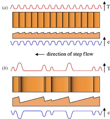
**Figure 17.** Step bunching on misaligned (111). Cartoon-like variations of the temperature ( $T$ ) and concentration ( $c$ ) are shown as examples of etchant inhomogeneities.
