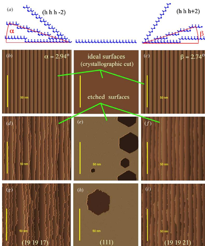
**Figure 15.** Different surface morphologies on misoriented (1 1 1) at medium concentration. Simulation.
