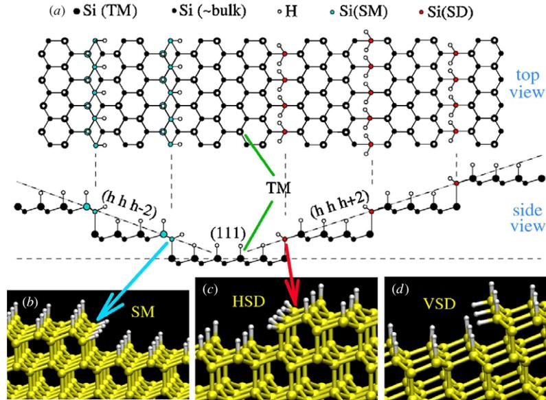
**Figure 6.** Identification of the typical surface sites appearing on (111).
