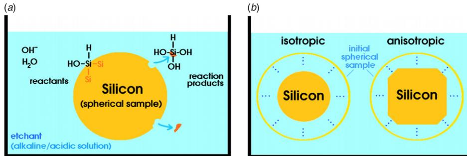
**Figure 1.** (a) Schematic illustration of the dissolution process during wet etching. (b) Wet etching can be isotropic or anisotropic. From [46] (figure 1).
