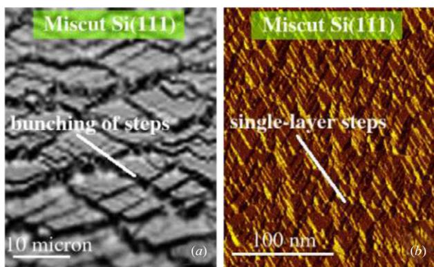
**Figure 16.** Step bunching on misaligned (1 1 1): (a) experiment (Sato Laboratory, Nagoya University, unpublished), (b) atomistic simulation.
