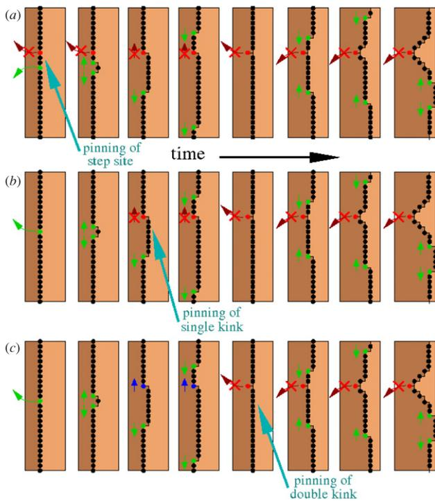
**Figure 13.** Schematic description of some convex tip pinning mechanisms on (1 1 1).
