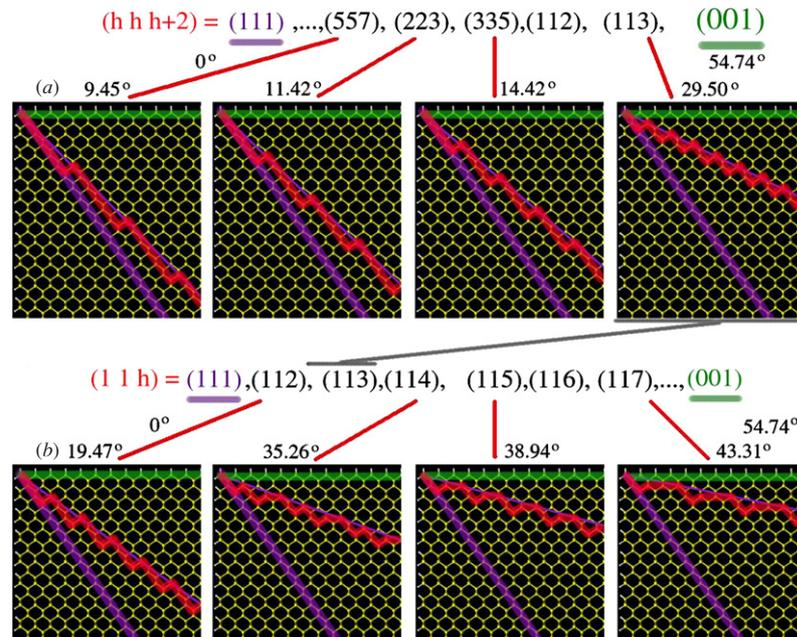
**Figure 34.** Crystallographic profile of the stepped surfaces between (1 1 1) and (1 0 0).
