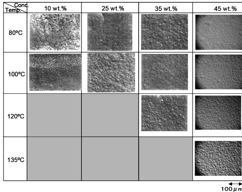
**Figure 26.** Morphology of (100) as a function of KOH concentration and temperature. Optical differential interference contrast. From [72] (p 20).
