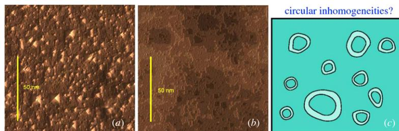
**Figure 27.** Simulated morphology of (1 0 0) with (a) and without micromasking (b). (c) Proposed shape of the etchant inhomogeneities on (1 0 0).
