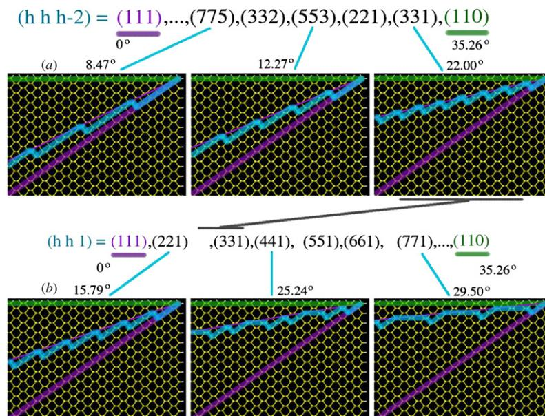
Figure 37. Crystallographic profile of the stepped surfaces between (111) and (110).
