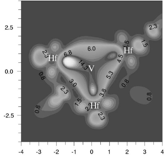
FIG. 10. Spin density in a plane containing three Hf ions neighboring the threefold-coordinated oxygen vacancy ( $V$ ) with one electron removed from the system. The charge density is in  $0.1e/\text{Å}^3$  and all distances are in Å.
