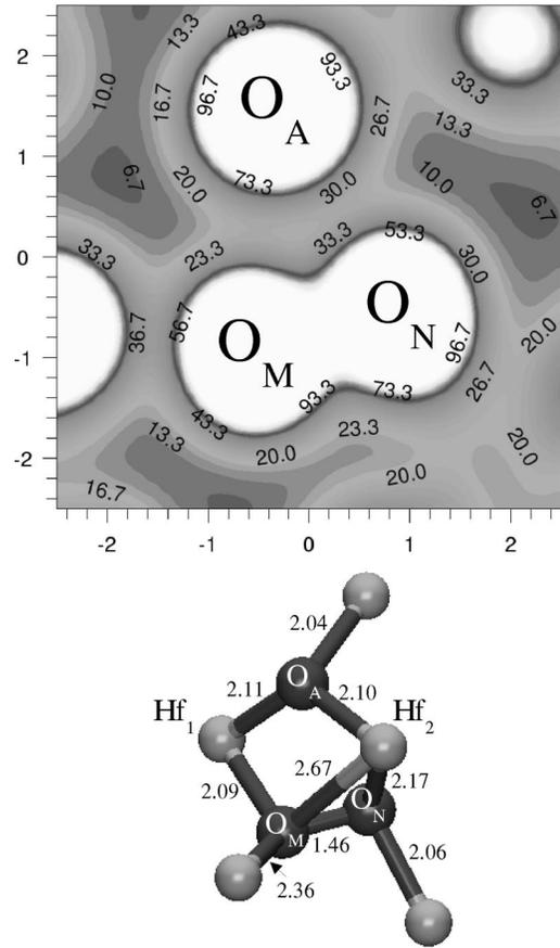
FIG. 9. Charge density and atomic structure of a doubly charged interstitial oxygen molecule ( $O_N$ - $O_M$ ) near a threefold-coordinated lattice oxygen site ( $O_A$ ). The charge density is taken in a plane through  $O_M$ ,  $O_N$ , and  $O_A$  in  $0.1e/\text{\AA}^3$  and all distances are in  $\text{\AA}$ .
