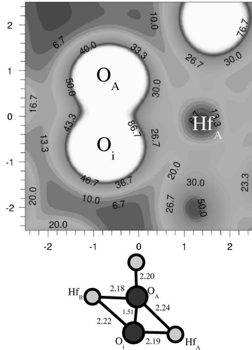
FIG. 3. Charge density in the plane through  $Hf_A$ ,  $O_A$ , and  $O_i$ , and a schematic diagram of neutral oxygen interstitial ( $O_i$ ) near a threefold-coordinated oxygen ( $O_A$ ) in hafnia. The charge density is in  $0.1e/\text{Å}^3$  and all distances are in Å.
