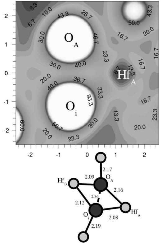
FIG. 5. Charge density in the plane through  $\text{Hf}_A$ ,  $\text{O}_A$ , and  $\text{O}_i$ , and schematic diagram of doubly charged oxygen interstitial ( $\text{O}_i$ ) near a threefold-coordinated oxygen ( $\text{O}_A$ ) in hafnia. The charge density is in  $0.1e/\text{\AA}^3$  and all distances are in  $\text{\AA}$ .
