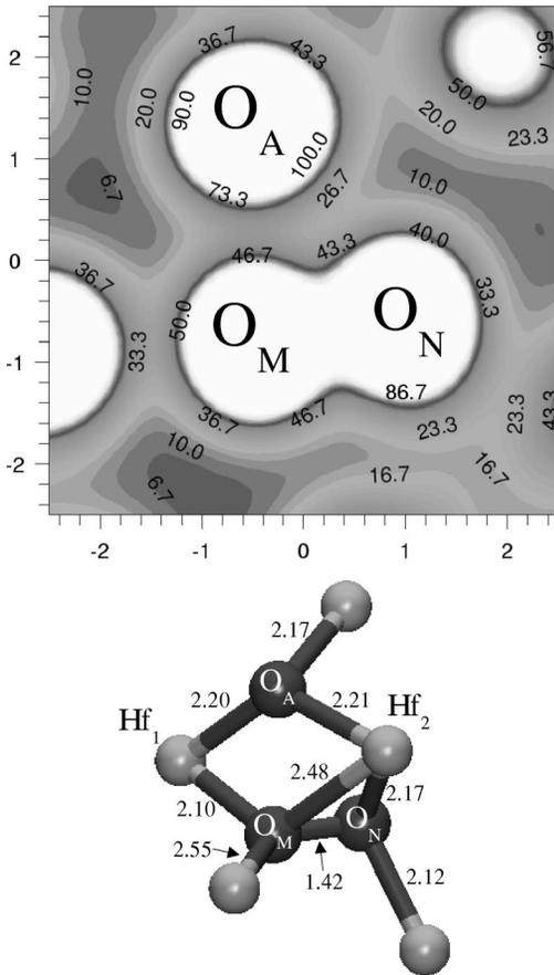
FIG. 8. Charge density and atomic structure of a singly charged interstitial oxygen molecule ( $O_N$ - $O_M$ ) near a threefold-coordinated lattice oxygen site ( $O_A$ ). The charge density is taken in a plane through  $O_M$ ,  $O_N$ , and  $O_A$  in  $0.1e/\text{\AA}^3$  and all distances are in  $\text{\AA}$ .
