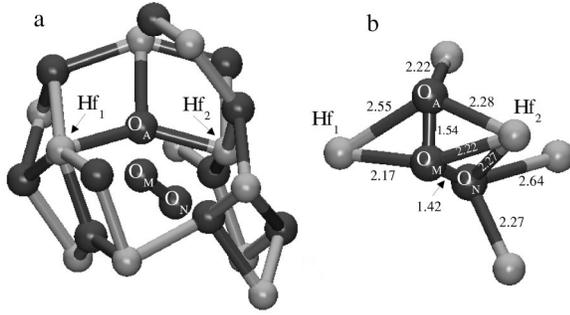
FIG. 6. (a) Atomic structure of ideal monoclinic hafnia with the neutral interstitial oxygen molecule ( $O_N$ - $O_M$ ) introduced near the threefold-coordinated lattice oxygen site ( $O_A$ ). (b) Close-up of the defect structure after relaxation. Equivalent atoms in the ideal and defected structure are labeled. All distances are in Å.
