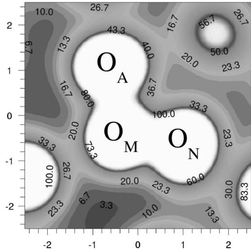
FIG. 7. Charge density of the neutral interstitial oxygen molecule ( $O_N$ - $O_M$ ) bonding with threefold-coordinated lattice oxygen site ( $O_A$ ). The charge density is taken in a plane through  $O_M$ ,  $O_N$ , and  $O_A$  in  $0.1e/\text{Å}^3$  and all distances are in Å.
