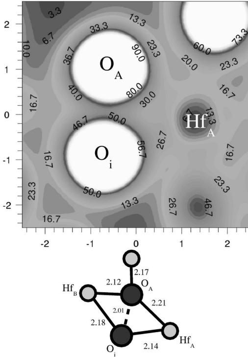
FIG. 4. Charge density in the plane through  $\text{Hf}_A$ ,  $\text{O}_A$ , and  $\text{O}_i$ , and schematic diagram of the singly charged oxygen interstitial ( $\text{O}_i$ ) near a threefold-coordinated oxygen ( $\text{O}_A$ ) in hafnia. The charge density is in  $0.1e/\text{\AA}^3$  and all distances are in  $\text{\AA}$ .
